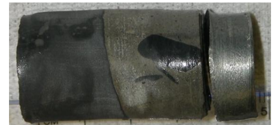
Figure 7: tpx-46-10-4005-xrd: Quartz is more abundant in formation side; an unassigned peak at 8.3, possibly corresponds to jennite; the formation side has calcite whereas the casing has very little; katoite is the dominant phase.
